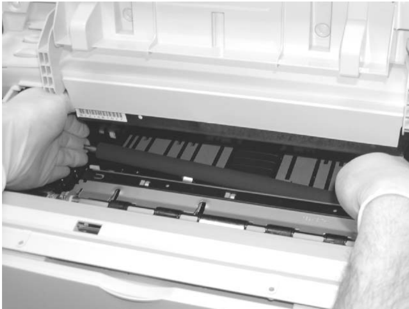
Transfer-roller assembly removal (3 of 3)
