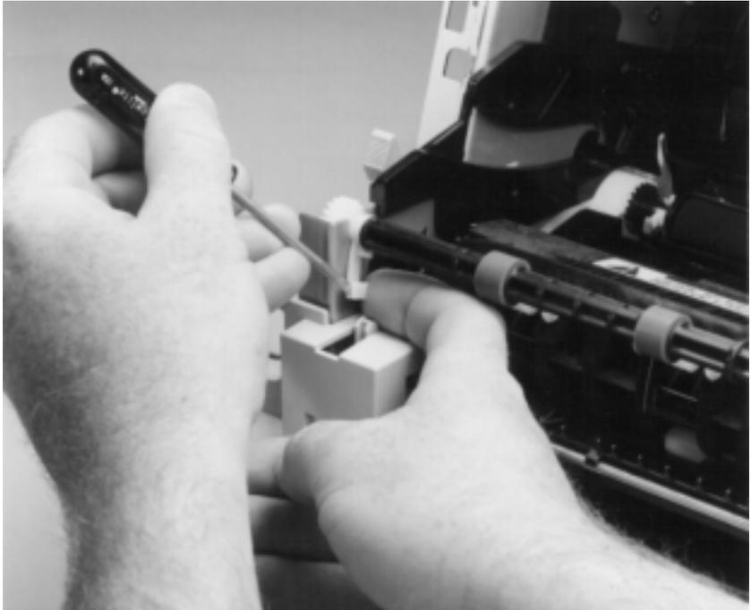
**Figure 39. Exit roller removal**
